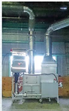
KESMAK KS6-4D Textile processing industry For odor/smoke emission 120m 3 /min
