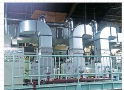
KESMAK KS40-4D × 3 units Textile processing industry For odor and gas emissions 40m 3 /min + Chemical injection system
